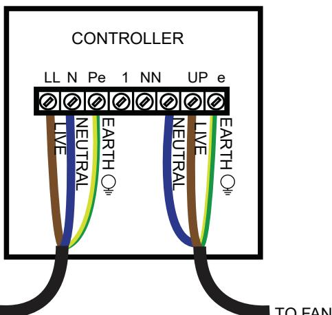
To install with thermostat fit thermostat switch in line on the live wire.
