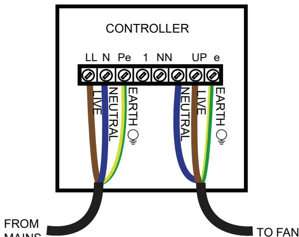
To install with thermostat fit thermostat switch in line on the live wire.
